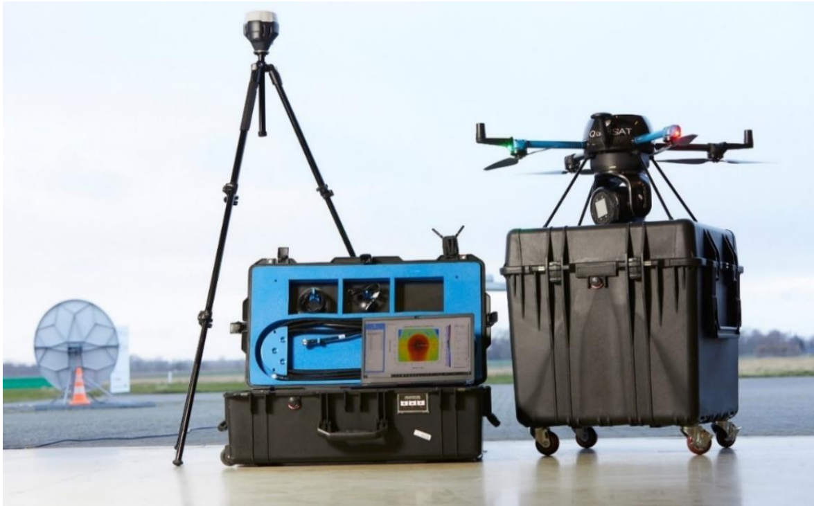
Figure 4: Example of a drone measuring system kit (courtesy of QuadSat).
